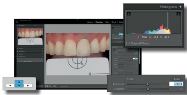
Fig 8 Measured L^*a^*b^* values are displayed below the histogram when the magnifying glass (cursor) is held steadily in position. Operating the up or down arrow keys on the keyboard adjusts image exposure. This is carried out until the known luminosity value ( L^*79 ) of the gray reference card has been replicated (ie, -0,12 ).
