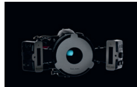
Fig 10: fluor_eyes filter mounted on Nikon R1C1 macro flash
